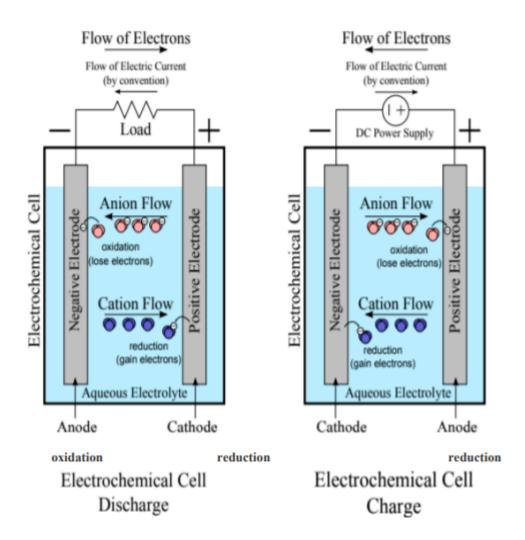
Charging and discharging cycle of an electrochemical battery cell. (Source: mdpi.com)
