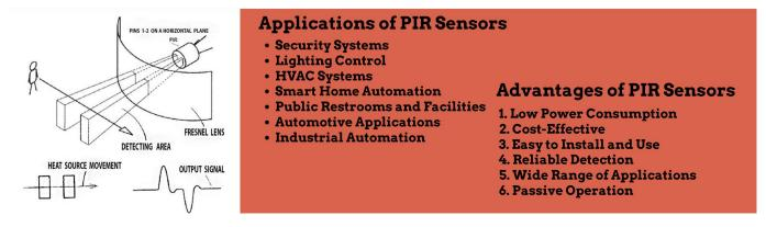
Passive Infrared (PIR) sensors are one of the most widely used motion detection technologies in the world today. They are crucial components in security systems, lighting controls, automatic doors, and various other applications where detecting movement is essential. But what exactly is a PIR sensor, and how does it work? This article provides a detailed exploration of PIR technology, its applications, advantages, and considerations when using PIR sensors.
